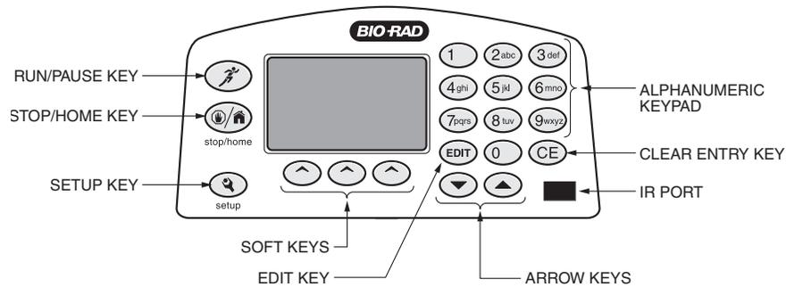
Fig. 4. Front Panel.
